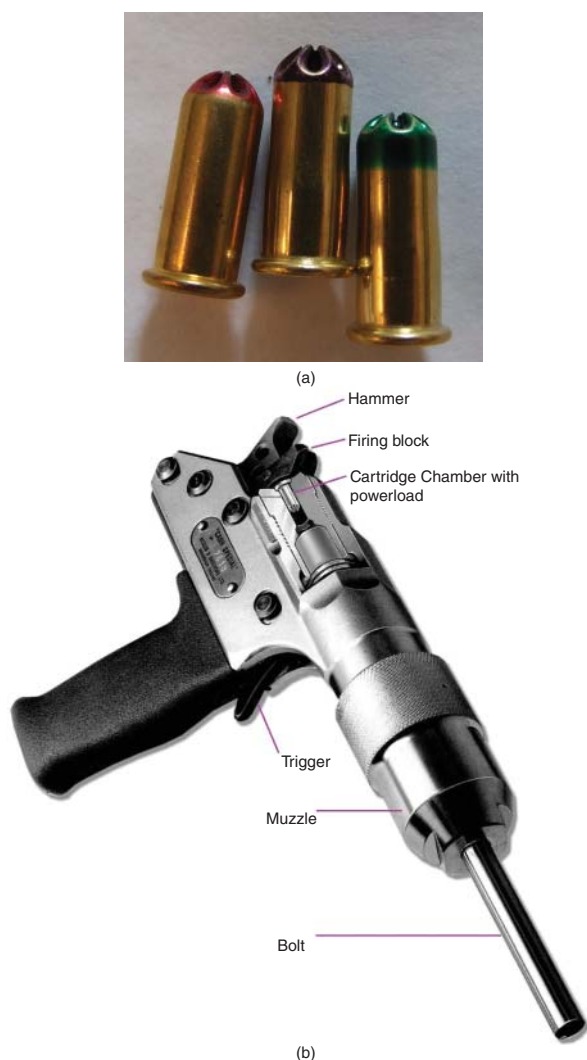
Figure 26.3 A CASH Special captive bolt gun (Reproduced courtesy of Accles & Shelvoke). (b) The bolt is shown extended for demonstration purposes. The inset (a) shows captive bolt cartridges in three power charges (from left to right: pink for calves, purple for heavy animals, green for bulls and very heavy animals).
